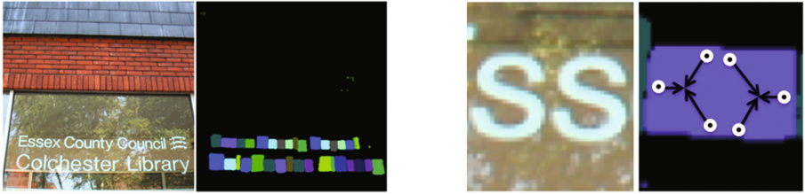
Fig. 4. Illustration of our network’s prediction. The left two images show the label prediction result on test image. As we can see, the prediction is very accurate. However, without other information, we can’t group pixels into characters, especially for those consecutive characters. The right two images show our goal of centroid prediction. With every pixel pointing to corresponding character’s centroid, we can easily accomplish instance segmentation for character. We also let our network to predict neighbor character’s centroid in order to combine characters into words. (Color figure online)
