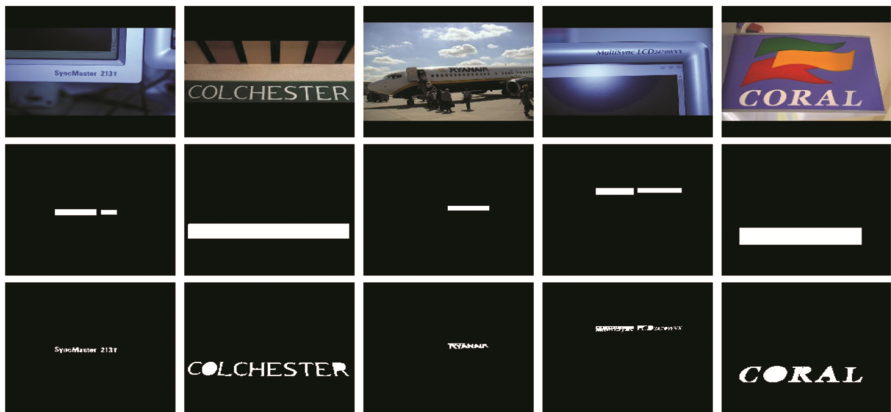
Fig. 3. Two types of ground truth mask. Original images are in the first row, the second and third rows contain bounding box ground truth masks and MSER ground truth masks.
